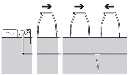
As the fault is approached, the Fault Find arrows will lock on to the signal and point forward and the dB readings will increase. When the fault is passed, the arrow will point back toward the fault.
