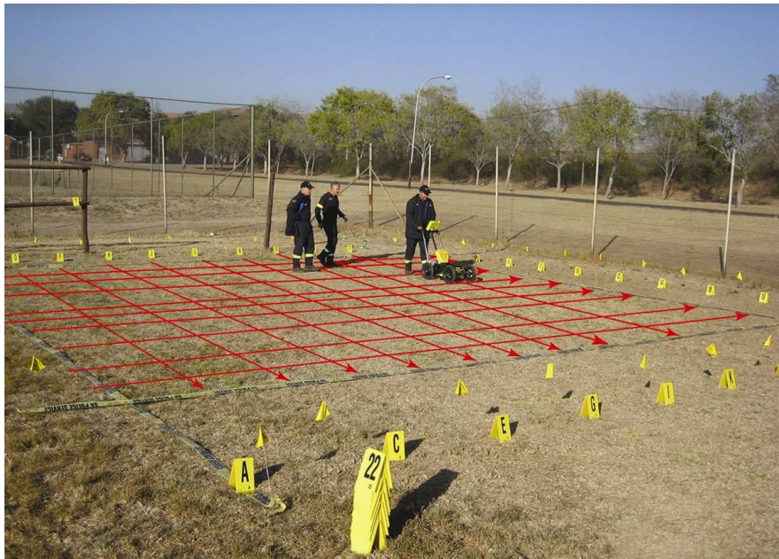
Figure 7-9: Example of a grid survey. The red lines are superimposed just to illustrate the concept.
