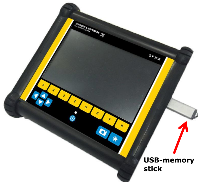
Figure 12-1: Insert a USB memory stick into the USB port on the Display Unit to export data.
